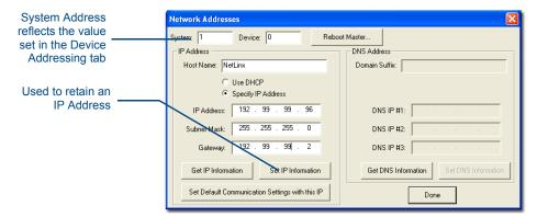
FIG. 22 Network Addresses dialog (for a pre-obtained Static IP Address)
